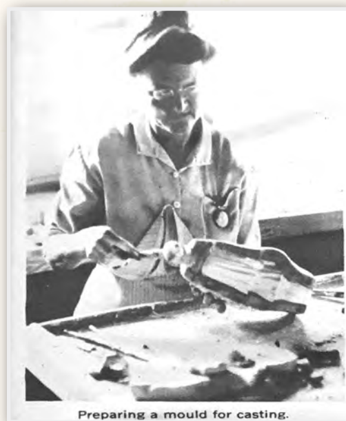
Preparing a mould for casting.
